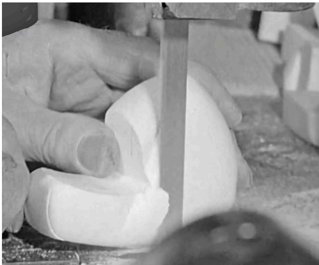
Fig. 2a-d. The main steps in the meerschaum pipe production process: (a) raw meerschaum blocks shaped into smaller pieces; (b) a turner behind his lathe; (c) a saw machine roughly shaping the blocks; and (d) a sculptor carefully shaping the meerschaum based on a specific design. (Pictures INA, Journal de Paris, 1966, film “Aux carrières d’écume”).
