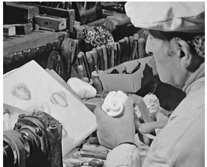
Fig. 2a-d. The main steps in the meerschaum pipe production process: (a) raw meerschaum blocks shaped into smaller pieces; (b) a turner behind his lathe; (c) a saw machine roughly shaping the blocks; and (d) a sculptor carefully shaping the meerschaum based on a specific design. (Pictures INA, Journal de Paris, 1966, film “Aux carrières d’écume”).
