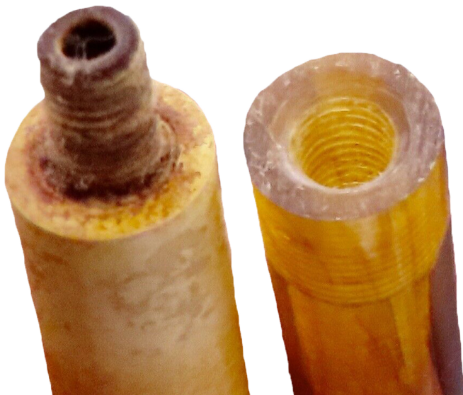
Fig. 10. Stem and bowl of a pipe equipped with the integrated thread.
